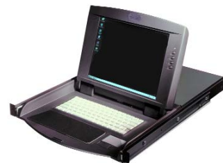
Rack-mount LCD with integrated KVM switch shown with included rack-mounting brackets and suspensions. The KVM sites directly behind the monitor so the entire unit only occupies 1U.
